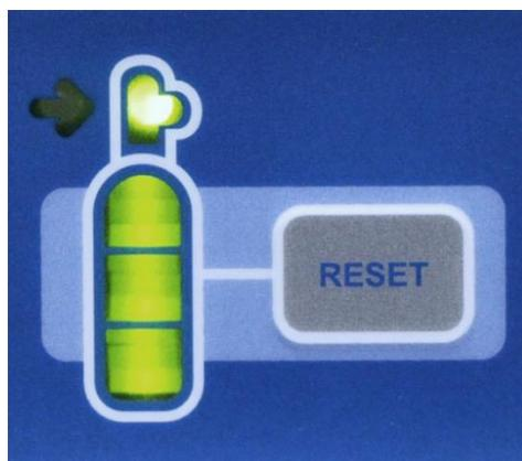
*Figure 12: N<sub>2</sub>O Gas Gauge RESET Button*
