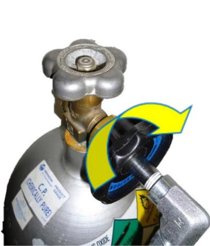
Figure 6: Attach Black Knob to Threaded Connection
