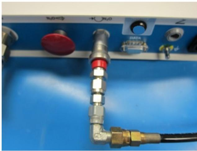
Figure 5: N<sub>2</sub>O Inlet Connection
