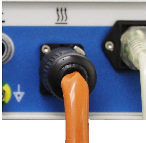
Figure 10: Plug Heater Band Cord into Receptacle
