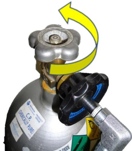
Figure 7: Turn Valve Counter-Clockwise to Open
