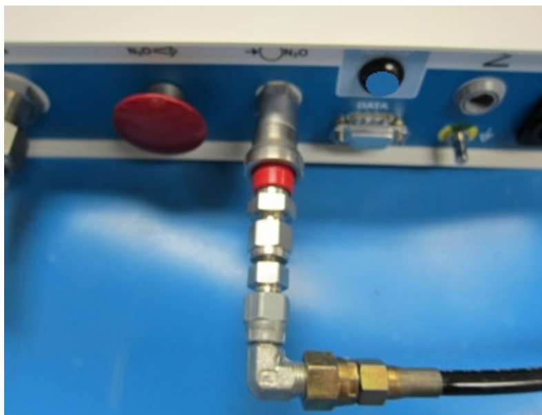
Figure 4: N 2 O Inlet Connection
