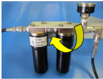
Figure 22: Filter Housing Removal
