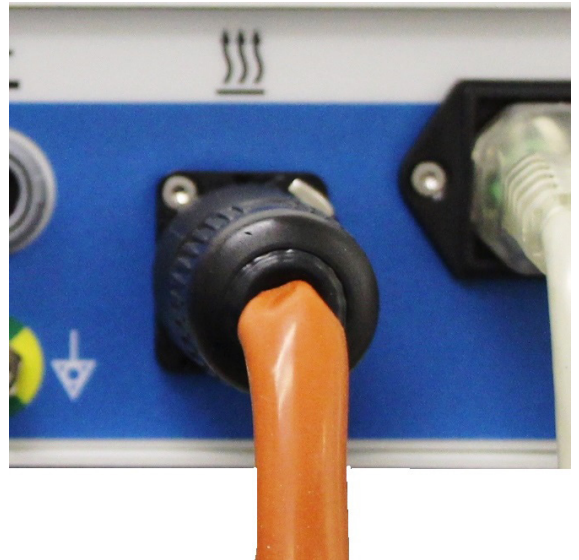
Figure 9: Plug Heater Band Cord into Receptacle
