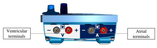
Figure 9: Lead connection terminals
