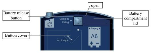
Figure 14: Battery compartment
